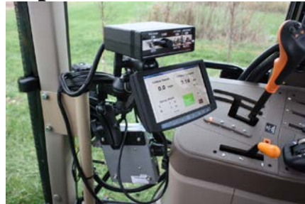
Touch screen and control box
